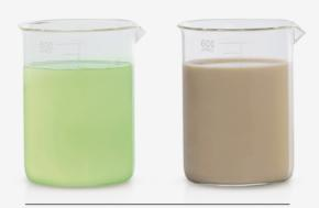
Comparative between the appearance of the Folia and the oil-based fluid after machining.
