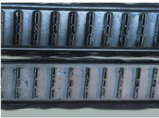
Deposit scaling on a radiator
