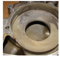
Cavitation in a waterpump (heavy duty application)
