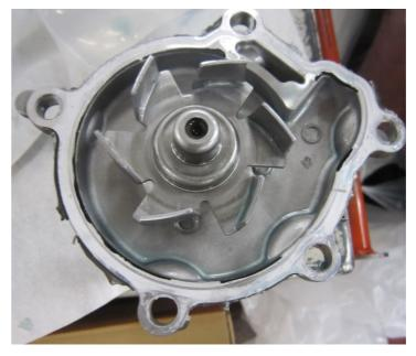
Picture: Waterpump after 65k KM field test(up), with P-OAT technology
